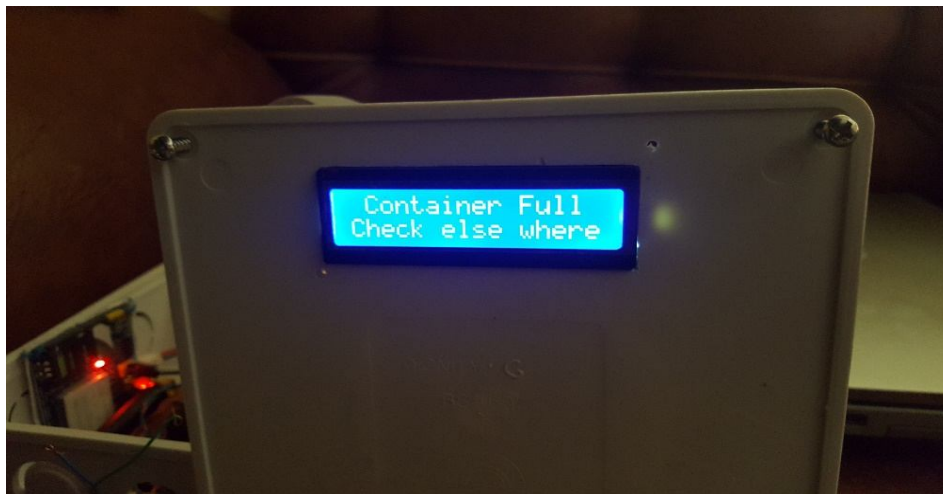
Fig. 7: Image view of the output unit displaying the current status of the system
