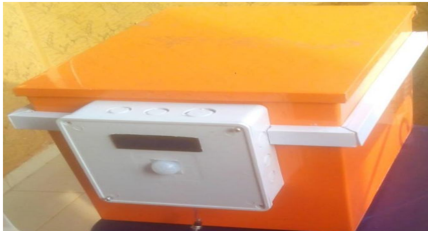
Fig. 11: Adaptable box fitted on the waste container
