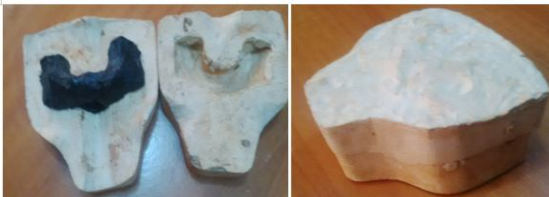
Fig. 6: Pattern Mould Box for the Connecting Rod Cap
