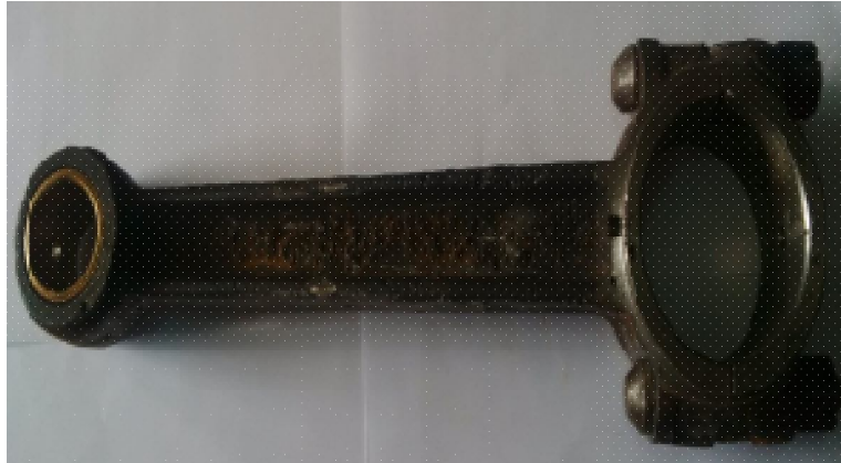
Fig. 10: Connecting Rod Produced from this Research Study
