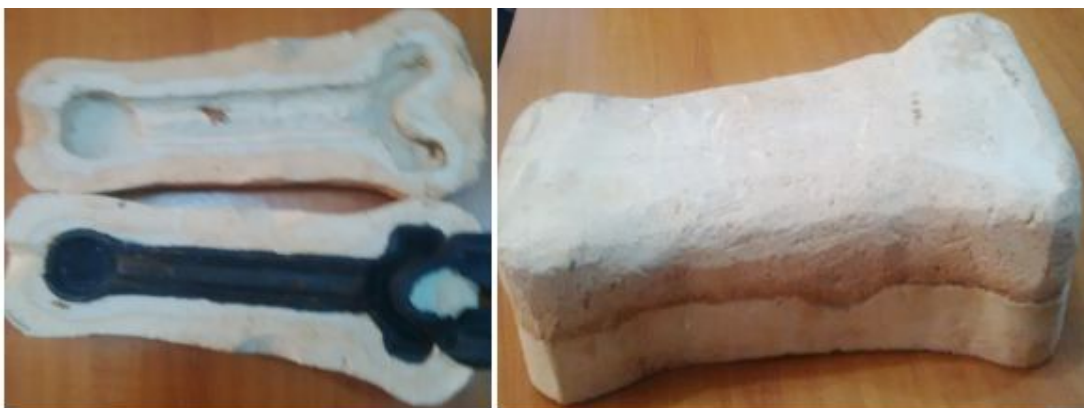
Fig. 5: Pattern Mould Box for the Connecting Rod
