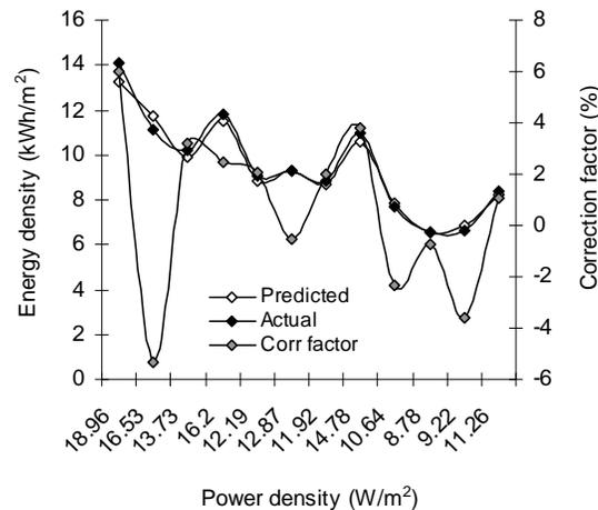
**Fig. 6: Variation of model-predicted energy density (relative to power density) with associated correction factor to actual result.**
