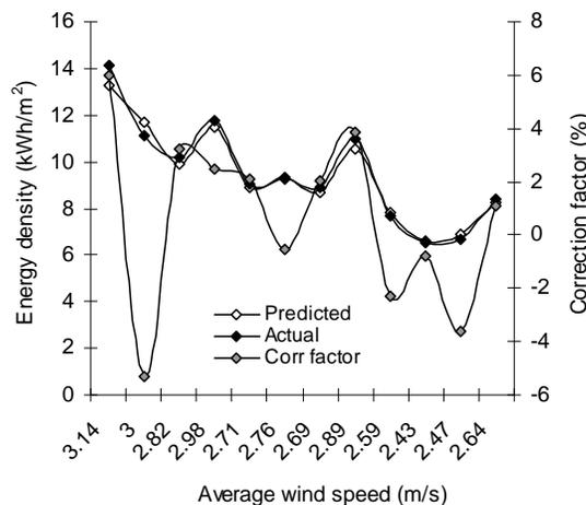
**Fig. 5: Variation of model-predicted energy density (relative to average wind speed) with associated correction factor to actual result.**
