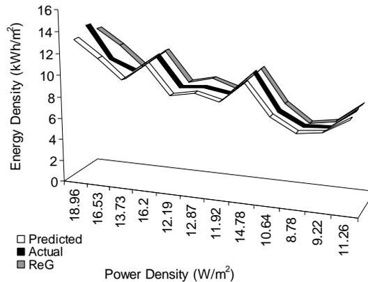
**Fig. 2: Comparison of the energy densities (relative to power density) as obtained from actual, predicted and regression results.**
