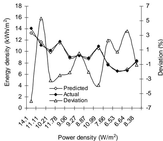
**Fig. 4: Variation of model-predicted energy density (relative to power density) with associated deviation from actual result**
