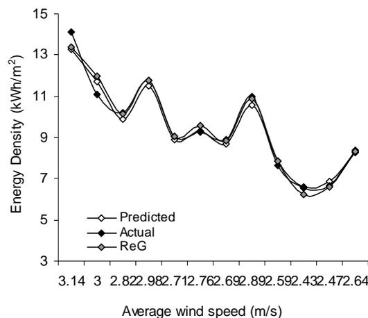
**Fig. 1: Comparison of the energy densities (relative to wind speed) as obtained from actual, predicted and regression results.**
