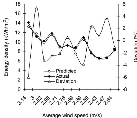
**Fig. 3: Variation of model-predicted energy density (relative to average wind speed) with associated deviation from actual result**
