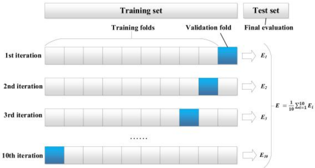
Fig.3: A 10-Fold Cross Validation method used to train, test and validate the selected machine learning modes for the prediction of PM2.5 Air pollutant levels within Awka Metropolis.
