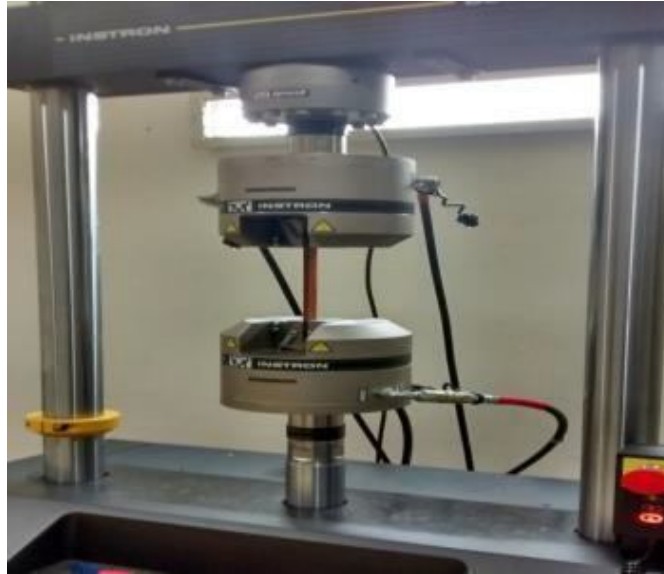
Fig.2: Hybrid fibre biodegradable composite sample subjected to tensile test
