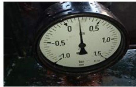
B: Precision Pressure Gauge
