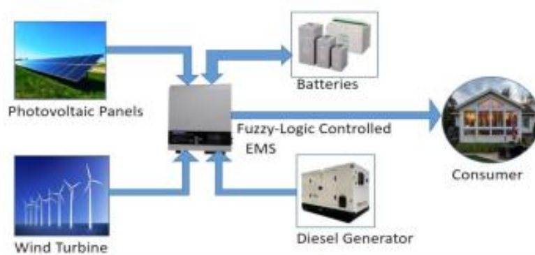
Fig 5: Hybrid renewable energy system structure.
