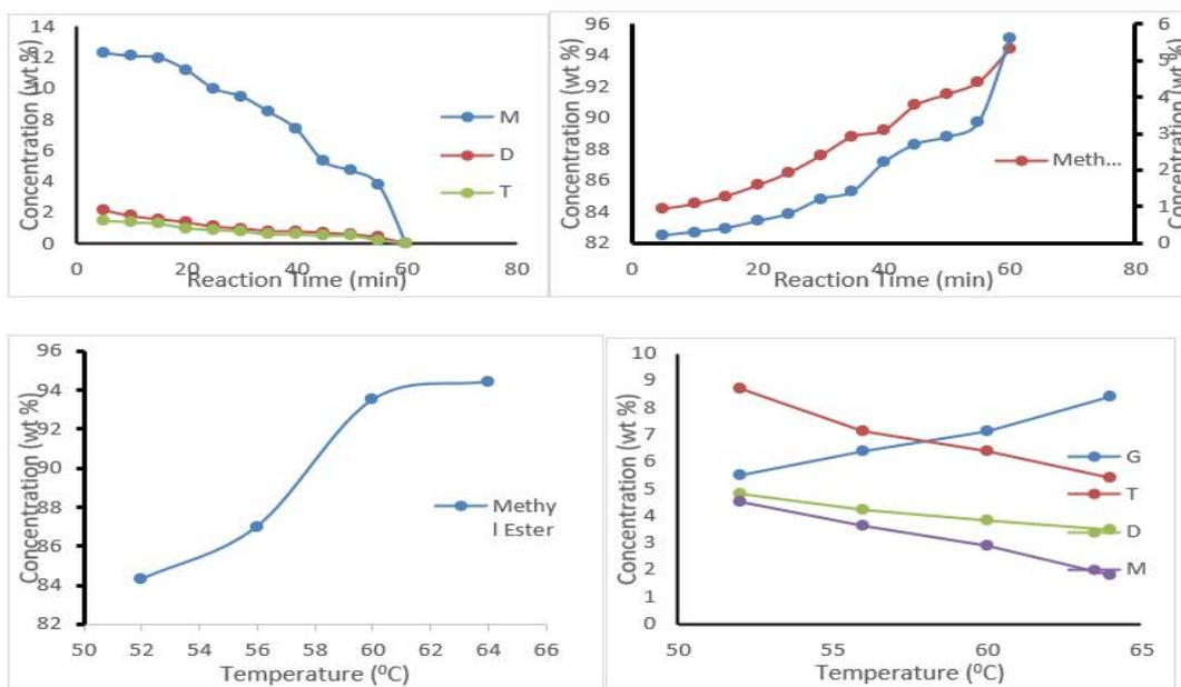
**Fig.6: Product distribution for trans-esterification of PFPO.**
