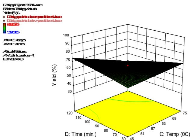
**Fig.4: Interaction effect of temperature and time on PFPOBD yield.**
