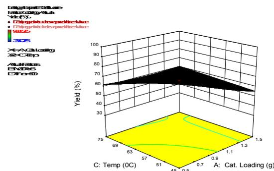
**Fig.2: Interaction effect of catalyst concentration and temperature on PFPOBD yield.**
