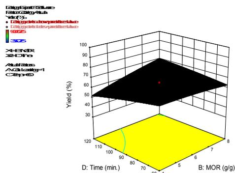
**Fig. 3: Interaction effect of methanol/oil molar ratio and time on PFPOBD yield.**
