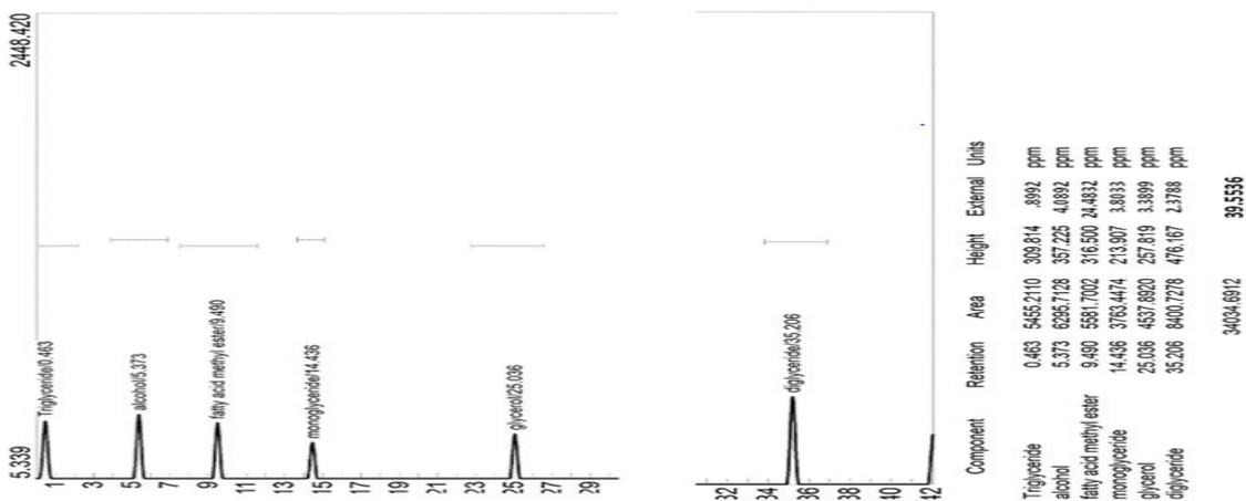
**Fig. 5: GCMS of purified fried palm oil biodiesel (PFPOBD)**
