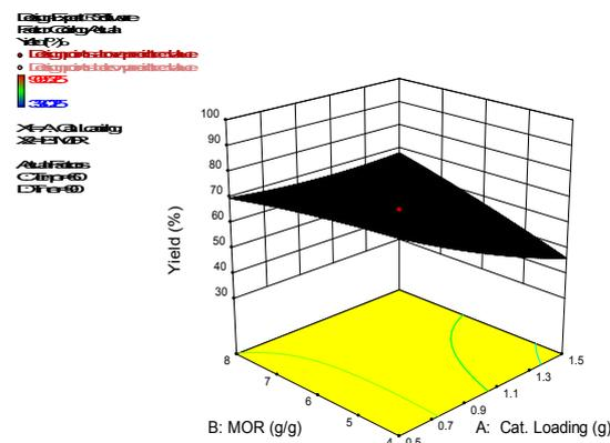
**Fig.1: Interaction effect of catalyst concentration and methanol/oil molar ratio on PFPOBD yield.**
