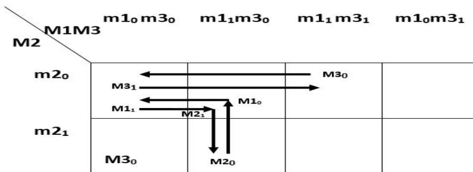
Fig. 6: Karnaugh maps for the printing sequence for the 3 cylinders (M1, M2, and M3), not optimized
