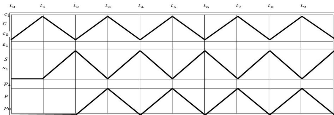
**Fig. 7: Displacement-step diagram for corking, stamping and palletizing cylinder actions**
