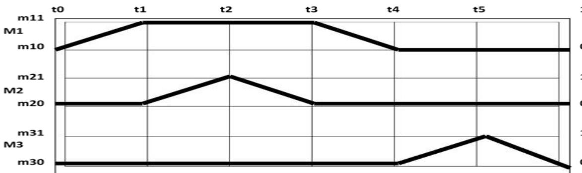
Fig. 5: Displacement-step diagram of the 3 cylinders
