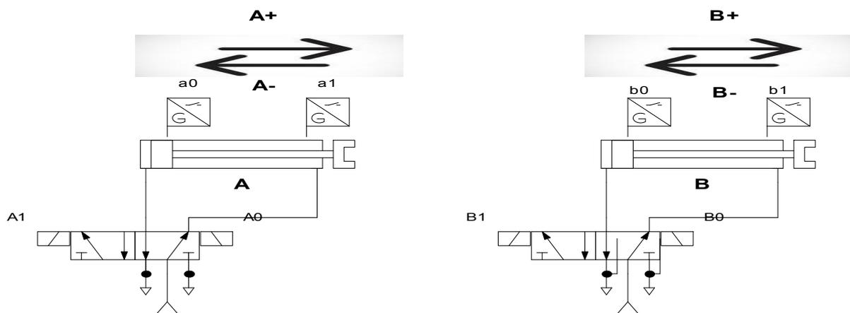
Fig. 3: Representation of variables for sequential movement of cylinders
