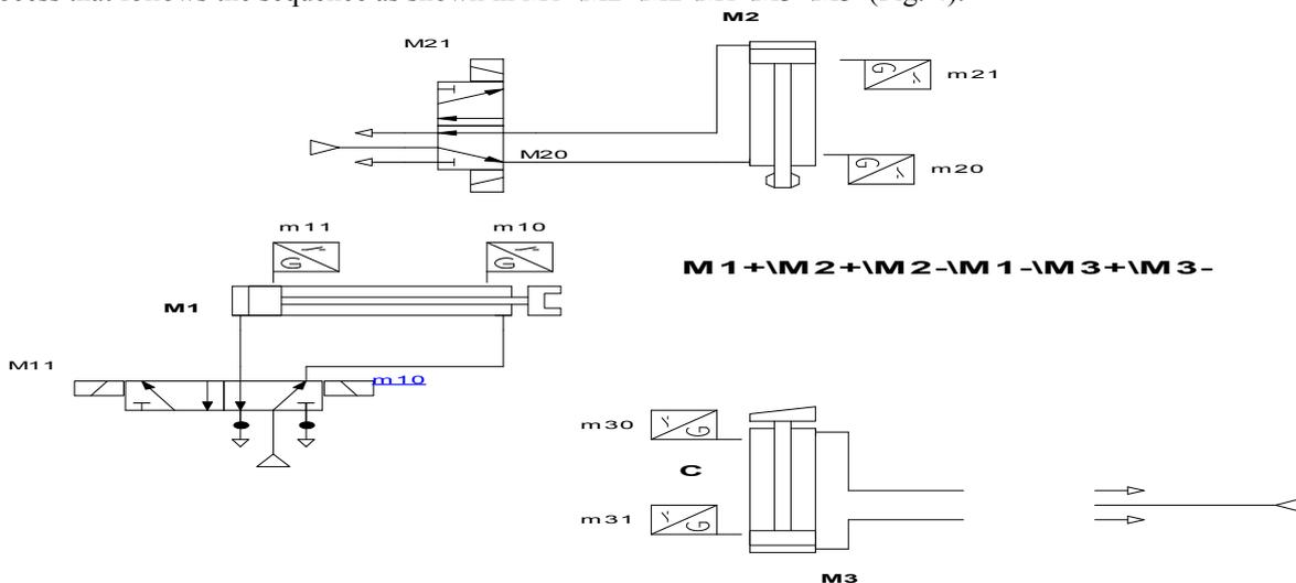
Fig. 4: Representation of the printing process on automation studio
