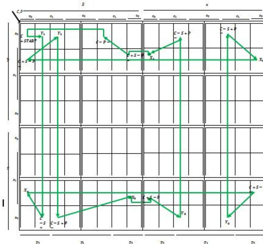
Fig. 9: K-map for corking, stamping and palletizing actions of the industrial automation process
