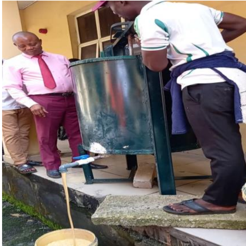
Fig.3: The paint mixer discharging paint after production
